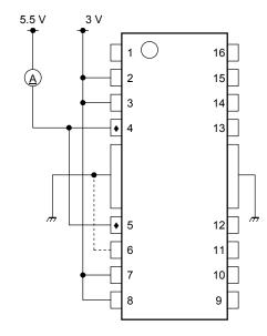
Note 1: The input logic of the heavy-load drive clock input pin (pin 6) is the same for High or Low.
