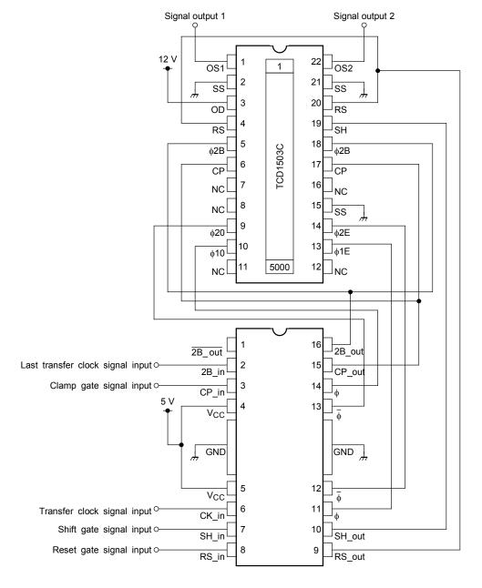
Note: Driving the CCD requires a lot of power. Toshiba recommends using a bypass capacitor connected to the 5 V power supply to stabilize voltage.
