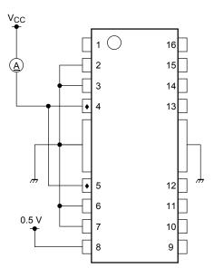
Note 2: When measuring input pins, connect the input pins that are not being measured to GND or power.
